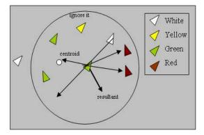
Fig. 3.1. Computing the direction of a green agent.
