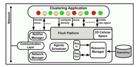
Fig. 4.2. The software architecture of P-Sparrow.
