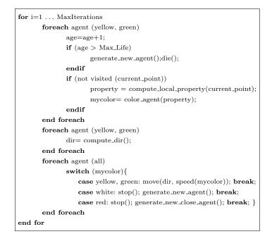
Fig. 3.2. The pseudo-code of the adaptive flocking algorithm.
