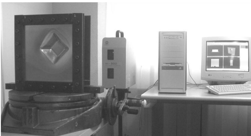
Figure 2.8. The laser based scanning system set-up.
