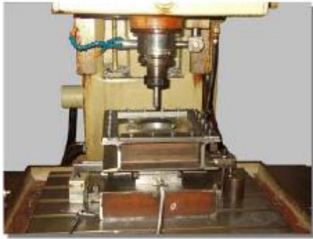
Figure 2.3. The ISF equipment for forces measurements on CNC machine.
