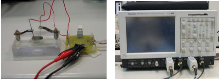
Fig.5.32. Picture of the circuit and electronics used to measure the macroscopic hysteresis loop.
