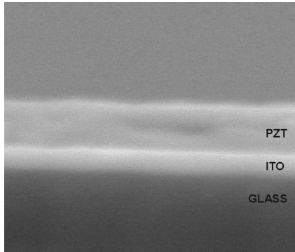
FIG. 1. Transversal section view of the thin PZT film deposited on ITO/glass.
