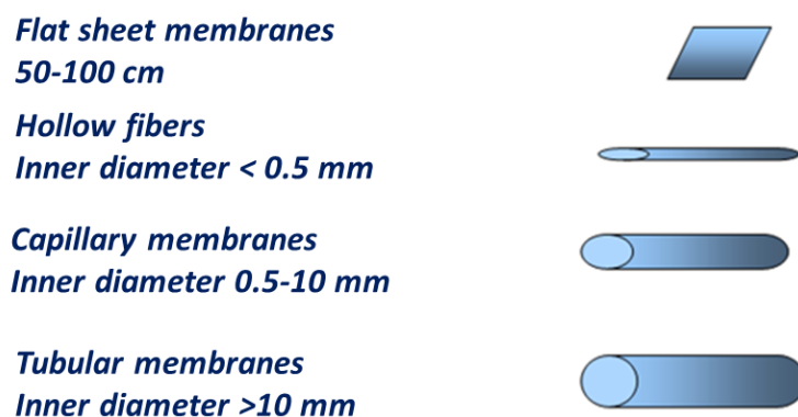
Figure 2.3. Schematic representation of typical membranes configuration. Readapted from [20].
