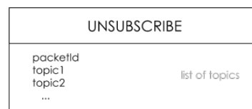
FIGURE 1.12: MQTT UNSUBSCRIBE packet structure
