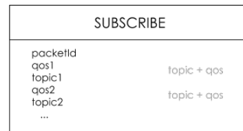
FIGURE 1.11: MQTT SUBSCRIBE packet structure
