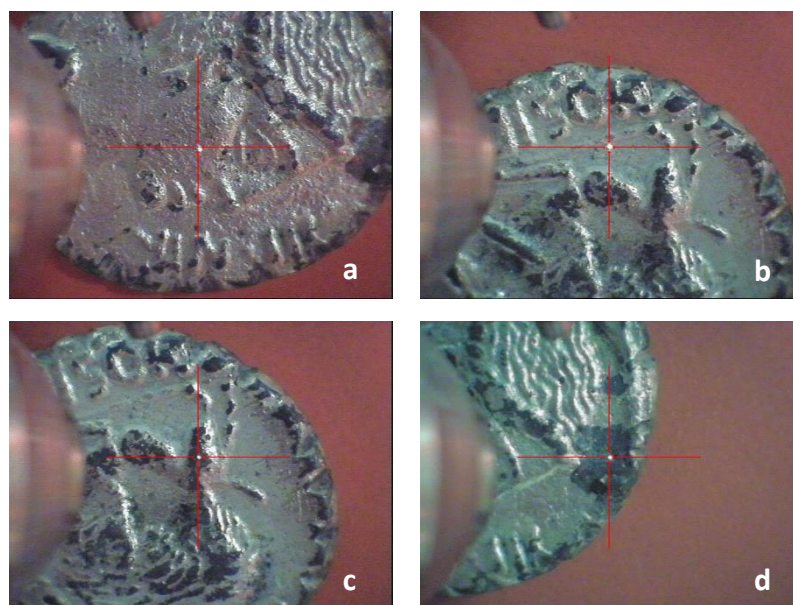
Figure 4.1.12: XRF measuring points on the M115 coin's silver layer (a-b) and flan (c-d)
