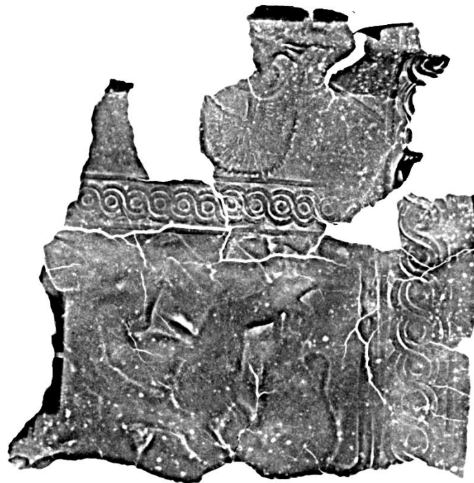
Figure 4.3.14: radiographic images of the bronze plaque analyzed using Gaussian Blur e Unsharp Mask filters
