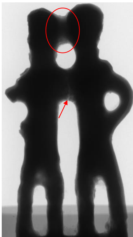
Figure 4.4.7: X-ray image in which the arrow indicates a lesion, while the circle highlights an area with less X-ray absorption_”type B”
