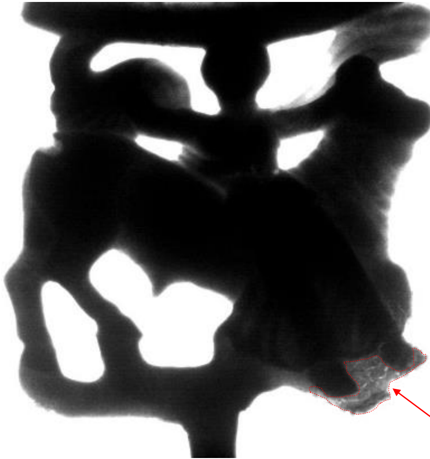
Figure 4.5.16: X-ray radiography of n. 142050 mirror in which the red arrows points to a less compact sample area
