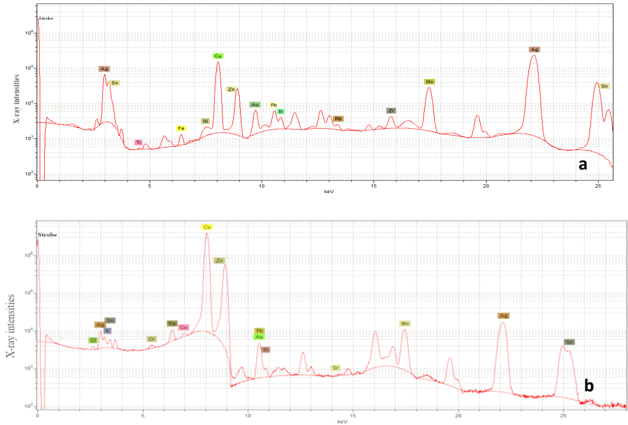
Figure 4.1.13: XRF spectra in logarithmic scale of the elements present on the M106 coin's silver layer (a) and flan (b)
