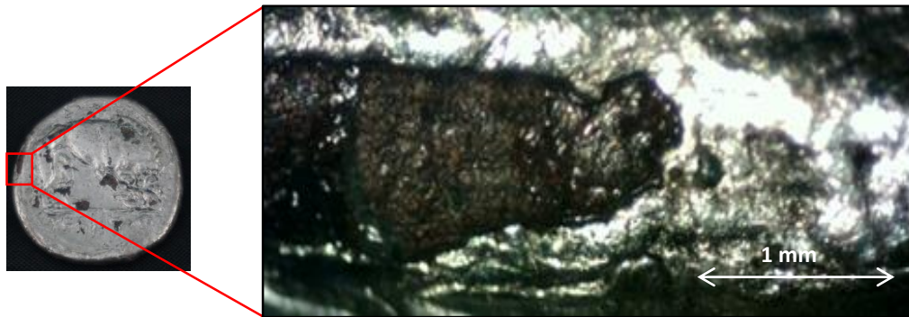
Figure 4.1.6: Detail from the edge of the M106 coin in which overlapping of silver layers is evident
