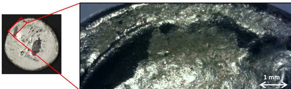
Figure 4.1.7: Detail of the obverse of the M114 coin showing the thinning of the silver layer
