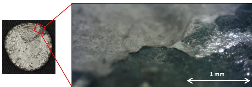
Figure 4.1.9: Detail of the obverse of the M115 coin pointing out the thinning of the silver layer and lifting of it from the substrate
