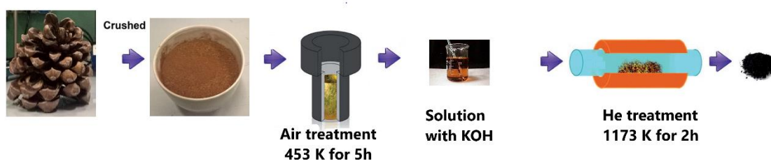
Figure 1. Schematic procedure for the preparation of the activated porous carbons from pinecones.
