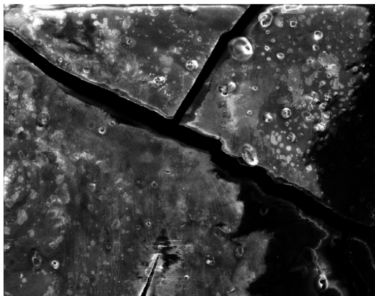
Figure 4. Overview of the DO3/39/7 sample surface (128x100 micron) showing the compactness of the material and the presence of few-micron wide spherules.
