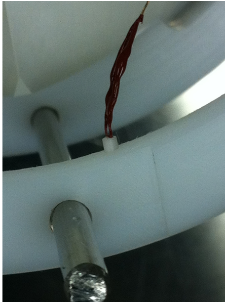
(a) Installing of 3 probes on the lower ring.
