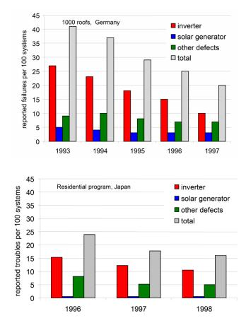
Figure 1.5: Figures show results of the large residential PV Program in Germany and Japan, presented by type of failure and failure frequency per 100 systems; data underline that the main failure source in PV plants is represented by inverter systems [19].
