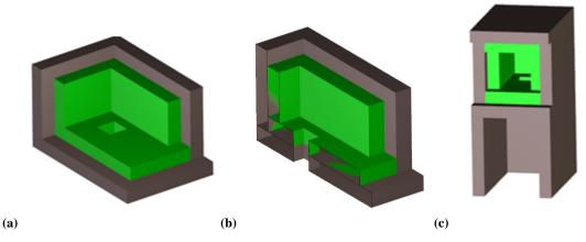
Figure 5.3: Figures represent the shielding thicknesses (a), the shielding section view (b) and the shielding whole structure (c); green is the 30% Borated PE, while grey is the Barite Concrete.
