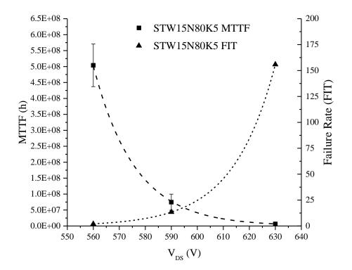
Figure 4.12: Failure parameters trend for a STW15N80K5 power MOSFET.
