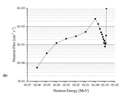
Figure 5.4: Figures show the D-D neutron spectrum (a) and the D-T neutron spectrum (b); the spectra have been evaluated using tally F4 in MCNP simulation in order to obtain the average neutron spectrum in a little spherical volume.
