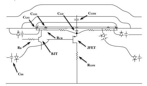
Figure 1.7: The figure shows the structure of the parasitic components in a power MOSFET device.
