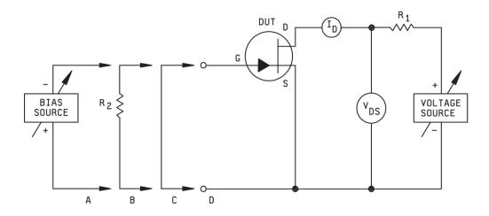
Figure 3.3: Figure represents the test circuit configurations for breakdown voltage characterisation suggested by Method 3407.1 of MIL-STD-750E [2].
