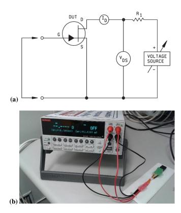
Figure 4.7: Figures show the gate-to-source short-circuit configuration used in DUTs characterisation (a) and the corresponding setup (b).
