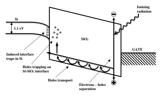
Figure 2.4: Figure shows the schematic energy band diagram for MOS structure with the major physical processes generating radiation-induced traps in Si-SiO<sub>2</sub> interface.
