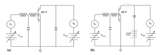
Figure 3.2: Figure shows the SEB/SEGR test circuit (a) and SEB circumvention and monitoring circuit (b) supplied by Method 1080 of MIL-STD-750E [2].
