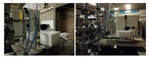
Figure 5.5: Figure shows the experimental setup with Li target and siloxane organic scintillator positioned at 26° with respect to the protons beam line; yellow disk is the beam stopper.
