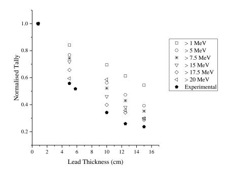
Figure 5.9: In figure is summarised the neutrons attenuation profile in function of lead thickness for different energy threshold.
