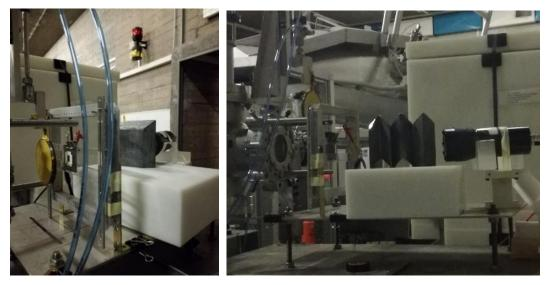
Figure 5.6: Figures shows experimental setup with lead bricks placed between the target and the neutron counter.
