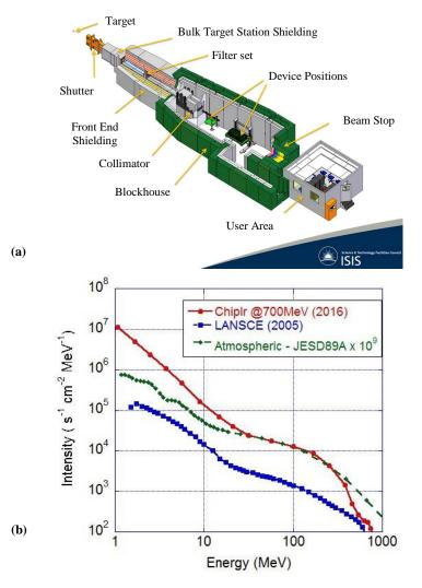
Figure 4.1: Figures shows ChipIr Neutron Irradiation Facility layout (a) and the ChipIr neutron spectrum in units of energy in comparison with the JESD89A atmospheric and LANSCE spectra (b) [1].
