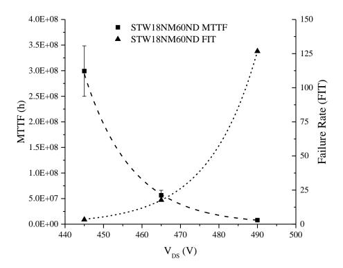
Figure 4.13: Failure parameters trend for a STW18NM60ND power MOSFET.
