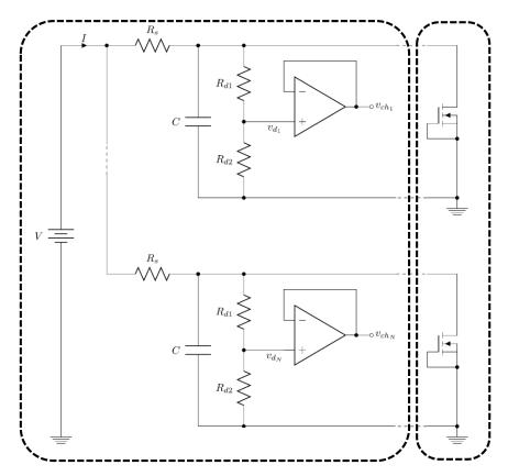
Figure 4.4: The figure represents the electronic layout of the capacitor board and op amp buffers (on left) and DUTs Board (on right).
