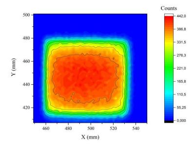
Figure 4.2: Figure shows a map of the neutron beam measured with a diamond detector [3].
