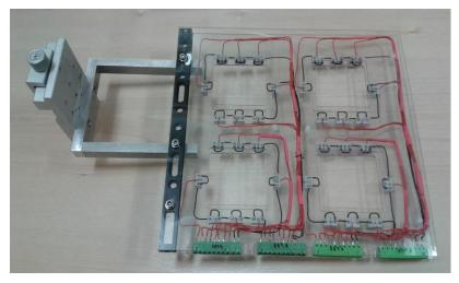
Figure 4.6: Figure shows the structure of DUTs Board.
