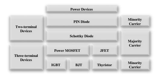
Figure 1.3: Power electronic devices groups with respect to the terminal number, on the right, and with respect to the carrier type, on the left.
