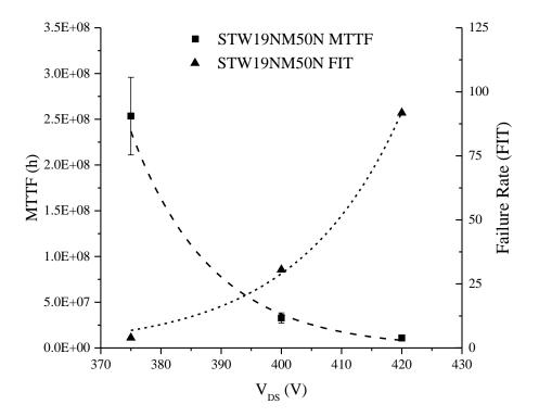
Figure 4.14: Failure parameters trend for a STW19NM50N power MOSFET.
