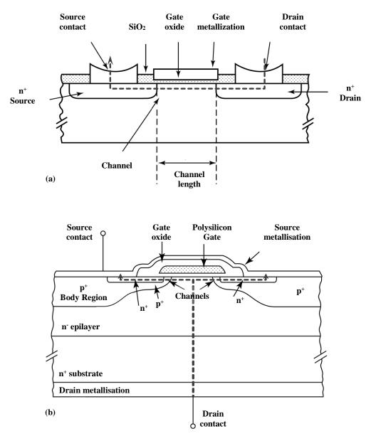
Figure 1.6: The figure illustrates Schematic diagram for (a) n-channel lateral MOSFET and (b) n-channel Power MOSFET [11; 16].
