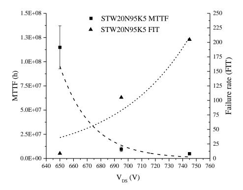
Figure 4.11: Failure parameters trend for a STW20N95K5 power MOSFET.
