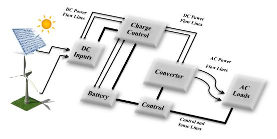
Figure 1.4: Figure shows a simplified diagram of a power system for the conversion of renewable sources of power [7].
