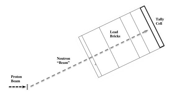
Figure 5.7: Figure represents the MCNP preliminary model of the experimental setup.
