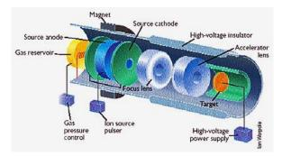
Figure 5.1: Figure shows the schematic design of a sealed-tube neutron generator with a Penning ion source.
