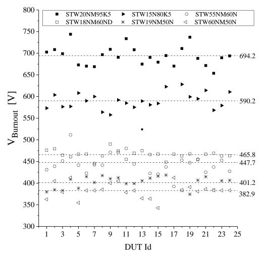
Figure 4.9: Figure summarises the SEEs thresholds evaluation in which symbols represent the devices V<sub>Burnout</sub> while dashed lines represent the mean V<sub>Burnout</sub> obtained for each type of device.
