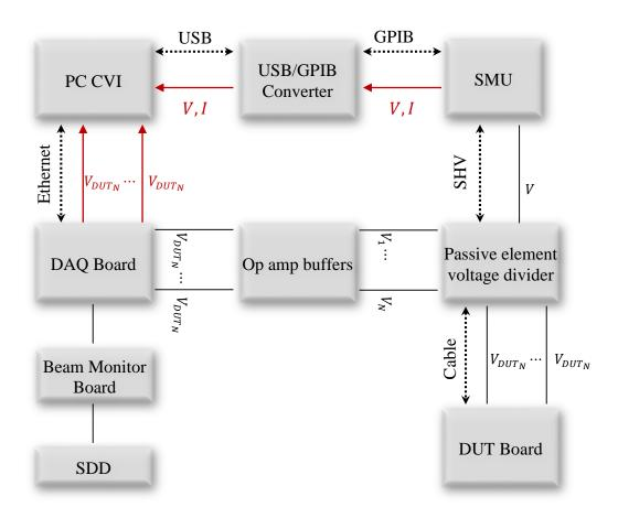
Figure 4.3: In figure are presented the block diagram of the experimental apparatus used during SEEs investigation.
