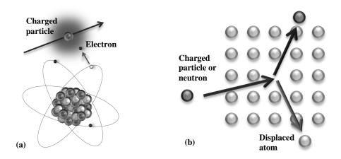
Figure 2.2: In figure are presented the mechanisms of radiation interactions; ionisation (a), in which Coulomb force due to energetic charged particles acts on the electrons surrounding atomic nuclei, and displacement (b), in which a charged particle or a neutron interact with atomic nuclei.
