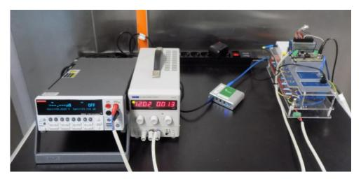
Figure 4.5: In figure the test equipment, from left, SMU, Beam monitor Board DC Supply and Capacitor Board.
