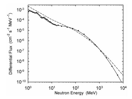
Figure 3.1: The differential flux of cosmic-ray-induced neutrons under reference conditions (sea level, New York City, mid-level solar activity, outdoors); the data points are the reference spectrum, the solid curve is the analytic fit to the reference spectrum, and the dashed curve is the model from the previous version of this standard [4].
