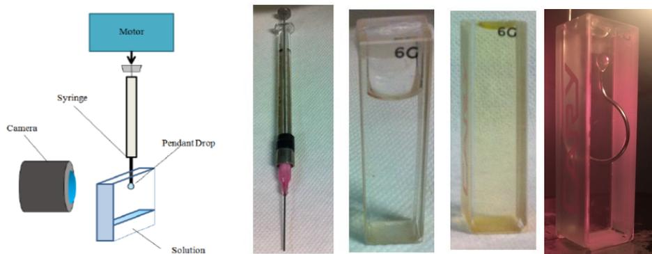
Figure 3.3.2 Syringe cuvette system schematization
