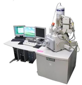
Fig. 26 Scanning Electron Microscope- FEI Quanta 200 Instrument
