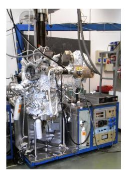
Fig. 4 Ultra-high vacuum chamber
