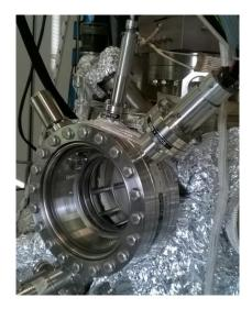
Fig. 8 LEED used for the experiments on this thesis
