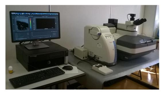
In our experiments a Thermo Fisher DXR Raman microscope with a 532 nm line was used.
