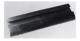
Figure 2.6. Stop mark defect, [100]
