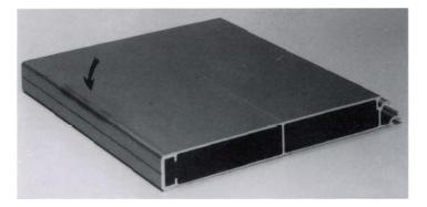
Figure 2.18. Spots defect, [100]
