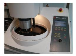
Figure 2.37. Tool utilized for grinding and polishing phases of the extruded specimen, in order to consequently analyze its microstructure
