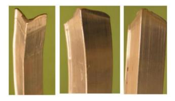
Figure 1.31. Distorted profile, faster material flow into the central zones, [50]
