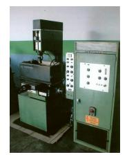
Figure 2.34. Electric discharge machine
