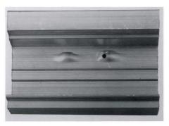
Figure 2.12. Deep blistering defect on the profile surface, [100]
