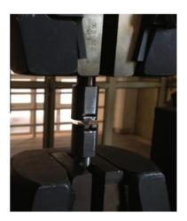
Figure 2.36. Clamping system utilized for tensile tests
