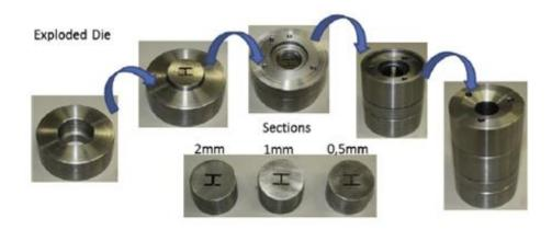
Figure 3.16. Exploded die used during the experimental campaign
