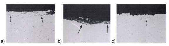
Figure 2.17. Streaks defect microstructure (500x) on an orthogonal plan to the defected surface, [100]
