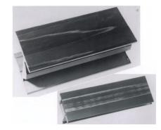
Figure 2.14. Bands or Streaks defect, [100]
