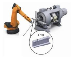
Figure 1.62. Curved extruded profile with variable cross section, [93]
