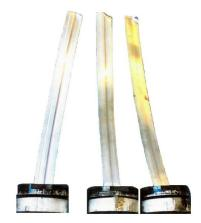
Figure 1.37. Comparison of the Profile 2 curvature, when applying a flat die (on the left), an intermediate pocket (in the middle) and a bigger pocket (on the right), [48]
