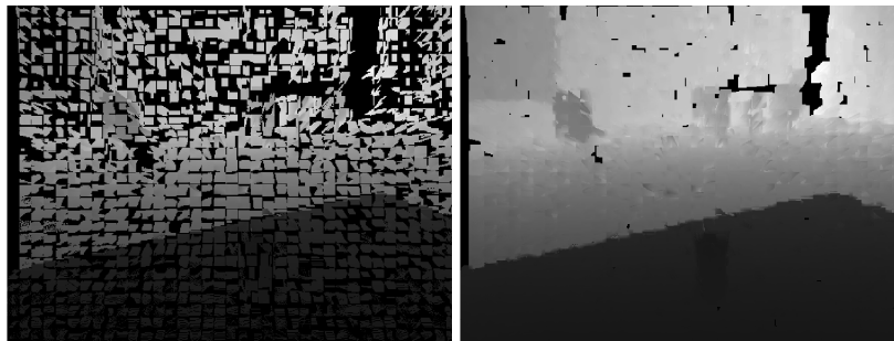
(d) Reconstructed image without hole-filling, surface blocks approximation (e) Reconstructed image with hole-filling, surface blocks approximation
