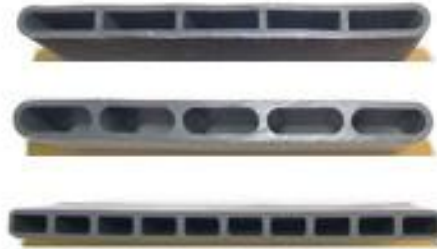
Fig. 1.9: Celle High Power Density (Fonte: Siemens Power Systems)
