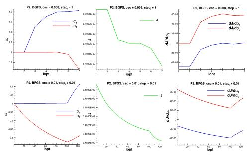
Figure 4.31: Behaviour of design variables (left column), cost function (middle column), and sensitivities (right column) versus the number of optimization cycles, using  $P_2$  elements.  $step_i = 1$  and csc = 0.008 (top row),  $step_i = 0.01$  and csc = 0.01 (bottom row).
