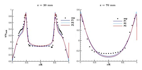
Figure 4.15: Comparison of numerical and experimental axial velocity inside the combustion chamber, at 20mm (right plot) and 70mm (left plot) from the cylinder head, using  $P_1$ ,  $P_2$  and  $P_3$  solutions.
