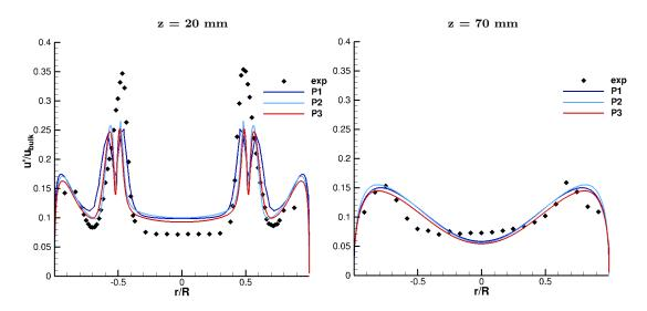
Figure 4.17: Comparison of numerical and experimental axial fluctuation velocity inside the combustion chamber, at 20mm (right plot) and 70mm (left plot) from the cylinder head, using  $P_1$ ,  $P_2$  and  $P_3$  solutions.
