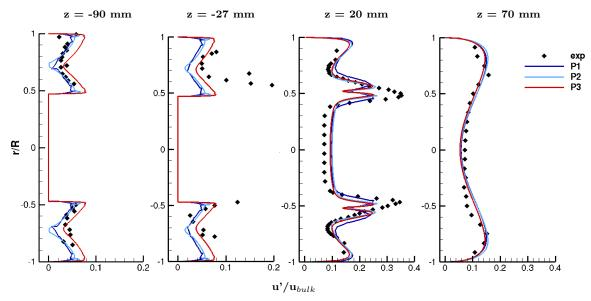
Figure 4.16: Comparison of numerical and experimental axial fluctuation velocity at -90mm, -27mm, 20mm, 70mm from the cylinder head, using  $P_1$ ,  $P_2$  and  $P_3$  solutions.
