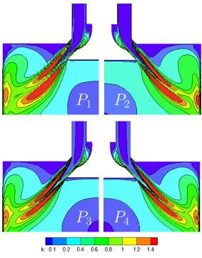
Figure 4.13: contours of the turbulent kinetic energy, k, close to the valve, for  $P_1$  (left column, first row),  $P_2$  (right column, first row),  $P_3$  (left column, bottom row) and  $P_4$  (right column, bottom row) elements.
