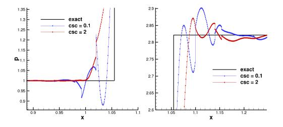
Figure 4.25: Undershoot and overshoot of pressure upstream (left plot) and downstream the shock (right plot). Exact solution versus  $P_5$  solutions computed along the y = 0.3 line using csc 0.1 and 2.
