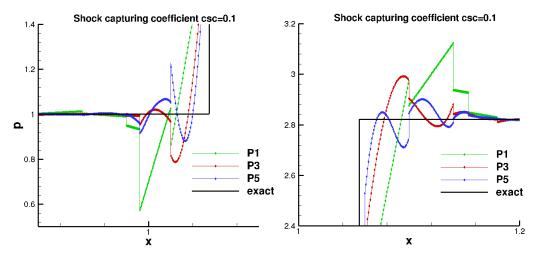
Figure 4.23: Undershoots and overshoots of the pressure upstream (left plot) and downstream (right plot) the shock. Exact solution versus approximate solutions computed along the y = 0.3 line using  $P_1$ ,  $P_3$  and  $P_5$  elements, with csc = 0.1.
