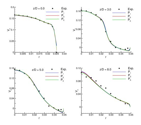
Figure 4.5: DG axial velocity profiles compared with the experimental data at the considered measurement stations: z/D = 0.0 and z/D = 3.0 (top row), z/D = 5.0 and z/D = 8.0 (bottom row).
