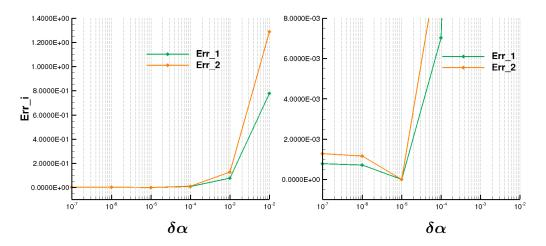
Figure 4.26: Behaviour of the differences between FD and AD sensitivities as a function of the perturbation step  $\delta \alpha$ , for csc = 0.1 and  $P_1$  elements (left plot) ,magnified view (right plot)
