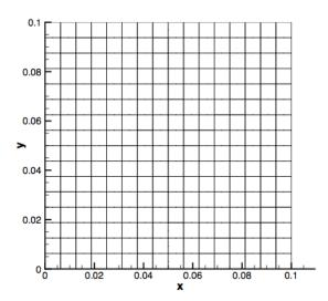
Figure 4.18: computational domain discretized with  $16 \times 16$  elements.
