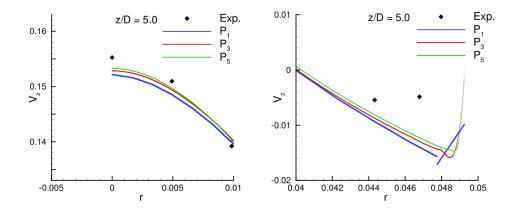
Figure 4.6: DG axial velocity profiles compared with the experimental data at z/D = 5.0, close-up near the axis (left column) and the wall (right column).
