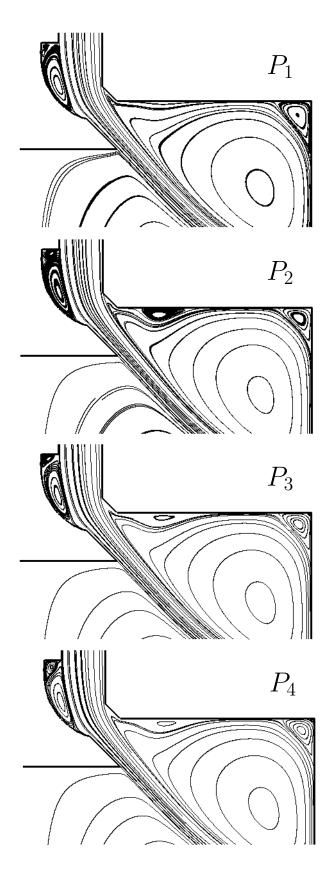
Figure 4.11: Magnified view of the streamlines close to the intake value, for  $P_1$  (first row),  $P_2$  (second row),  $P_3$  (third row) and  $P_4$  (fourth row) elements.
