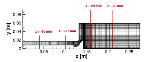
Figure 4.9: Computational grid upstream and downstream the valve, including measurement stations.
