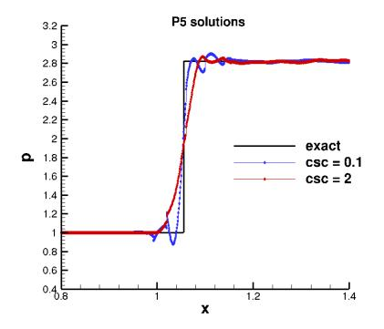
Figure 4.24: Comparison between exact and  $P_5$  solution along the y = 0.3 line, for csc = 0.1 and 2.
