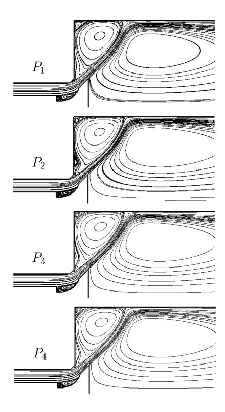
Figure 4.10: Streamlines along the intake valve and inside the cylinder, for  $P_1$  (first row),  $P_2$  (second row),  $P_3$  (third row) and  $P_4$  (fourth row) elements.
