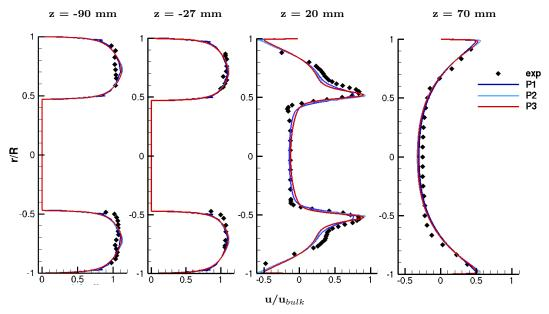
Figure 4.14: Comparison of numerical and experimental axial velocity at -90mm, -27mm, 20mm, 70mm from the cylinder head using  $P_1$ ,  $P_2$ ,  $P_3$  solutions.
