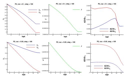
Figure 4.28: Behaviour of design variables (left column), cost function (middle column), and sensitivities (right column) versus the number of optimization cycles, using  $P_2$  elements and an initial step size of 100. csc = 0.1 (top row) and csc = 0.05 (bottom row).
