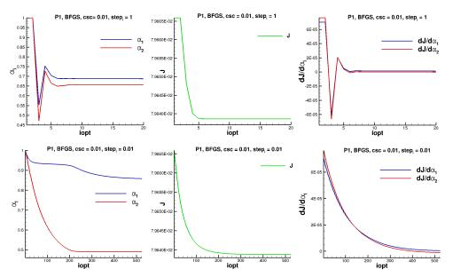
Figure 4.30: Behaviour of design variables (left column), cost function (middle column), and sensitivities (right column) versus the number of optimization cycles, using  $P_1$  elements and csc = 0.01.  $step_i = 1$  (top row),  $step_i = 0.01$  (bottom row).
