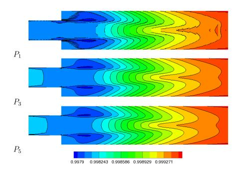
Figure 4.3: Contours of pressure obtained using  $P_1$  (top row),  $P_3$  (middle row) and  $P_5$  (bottom row) elements.
