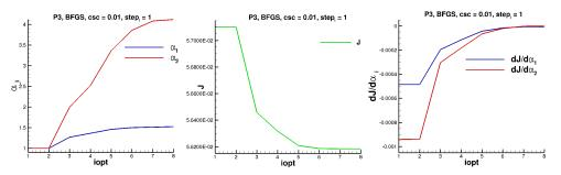
Figure 4.32: Behaviour of design variables (left column), cost function (middle column), and sensitivities (right column) versus the number of optimization cycles, using  $P_3$  elements,  $step_i = 1$ , csc = 0.01.
