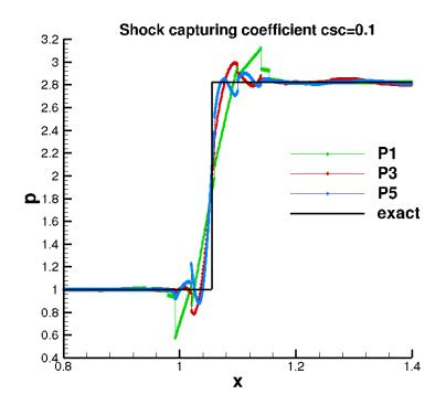
Figure 4.22: Comparison between exact and  $P_1$ ,  $P_3$  and  $P_5$  solutions, along the y = 0.3 line, using csc = 0.1.
