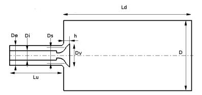
Figure 4.8: Detailed view of the geometry of the engine head
