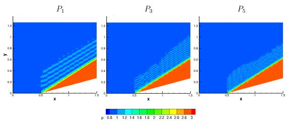
Figure 4.21: Pressure contours for  $P_1$  (left plot),  $P_3$  (middle plot) and  $P_5$  elements (right plot), using csc = 0.1.
