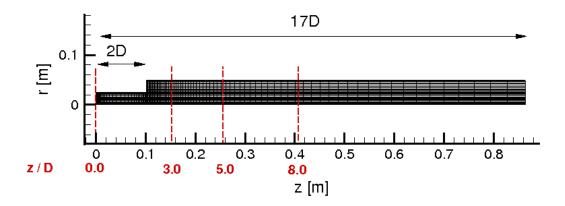
Figure 4.1: Computational grid for the abrupt axisymmetric expansion test-case, including measurement stations.
