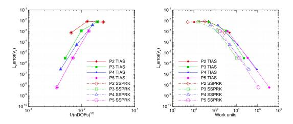
Figure 4.19:  $L_2 \operatorname{error}(u)$  as a function of  $1/\sqrt{nDOFs}$  (left) and work units (right).
