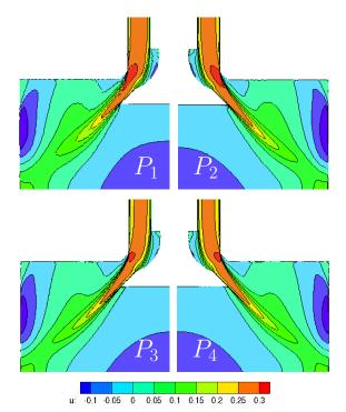
Figure 4.12: contours of the axial velocity, u, close to the valve, for  $P_1$  (left column, first row),  $P_2$  (right column, first row),  $P_3$  (left column, bottom row) and  $P_4$  (right column, bottom row) elements.
