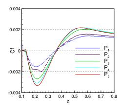
Figure 4.7: Skin friction coefficient  $C_f$  along the wall of the duct, for  $P_1$ ,  $P_2$ ,  $P_3$ ,  $P_4$  and  $P_5$  elements.
