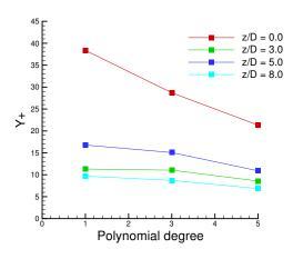
Figure 4.2:  $y^+$  values for the first cell-centroid  $y_1$  as a function of different polynomial degrees at the considered measurement stations.
