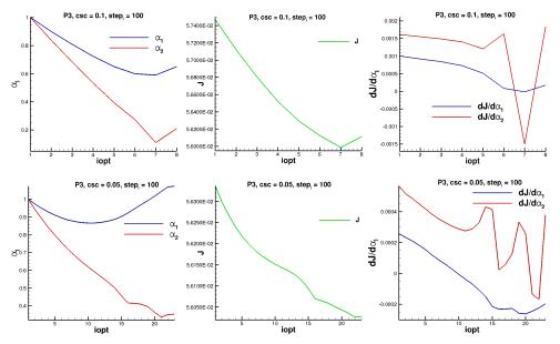
Figure 4.29: Behaviour of design variables (left column), cost function (middle column), and sensitivities (right column) versus the number of optimization cycles, using  $P_3$  elements and an initial step size of 100. csc = 0.1 (top row) and csc = 0.05 (bottom row).
