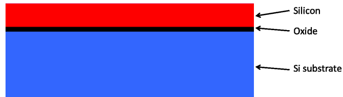
Figure 3.16: Initial SOI structure
