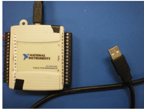
Figure 4.3: The data acquisition card used to acquire and generate voltages in the present design
