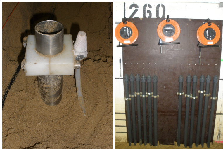
(a) Pressure cell of the piezometer (b) PVC pipes of piezometers and freetmeters
