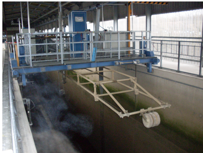
Figure 4.30: Beach profiler mounted on the carriage
