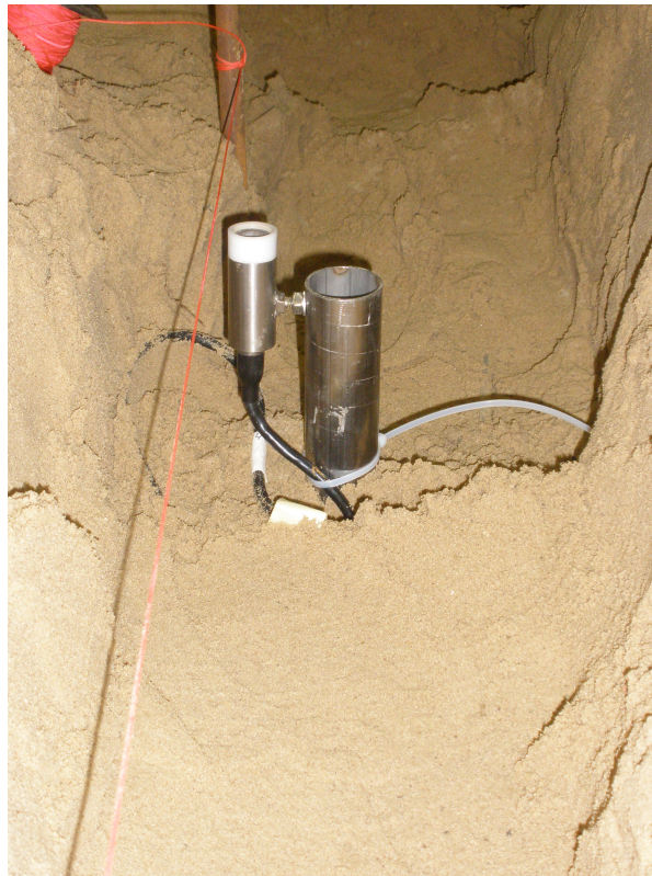
Figure 4.23: Pore pressure transducer inside the sand
