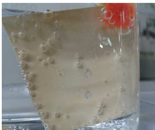
Figure 5.8.3 Oxygen formation at surface of PBM membrane with AUTEAB-RuPOMs nanoparticles in contact with H 2 O 2
