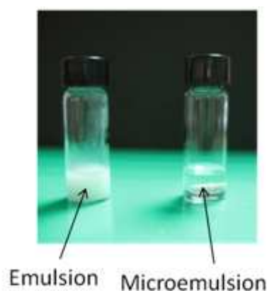
Figure 4.2.2 Optical appearance of an emulsion and a microemulsion
