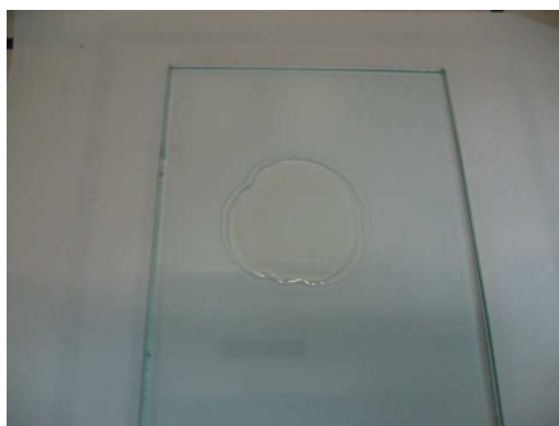
Figure 4.2.3 Optically transparent PBM after polymerization
