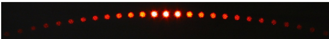
Fig 3.16 Photo of the diffraction pattern produced by the grating in the planar-planar periodic configuration.
