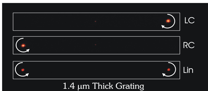
Fig 3.9 Diffraction patterns produced by the grating for 1.4\mu m cell thick in the wedge cell. LC: left circular polarization state of the impinging beam; RC: right circular polarization state of the impinging beam; Lin linear polarization state of the impinging beam.
