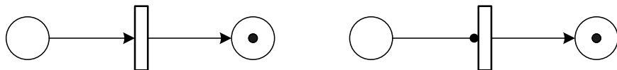
Figure 1.3: Petri Nets notation. On the left the classic Petri Net components, on the right an example of Petri Net with an inhibitor arc.
