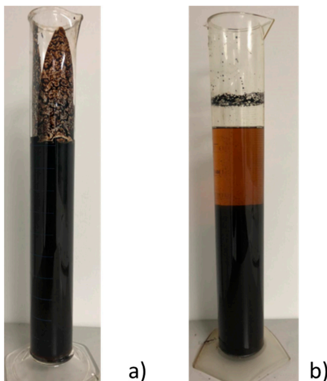
Figure 4. Pictorial representation of Alma bitumen emulsions obtained with liquid pitches (LP) additive (a), and without LP additive (b).
