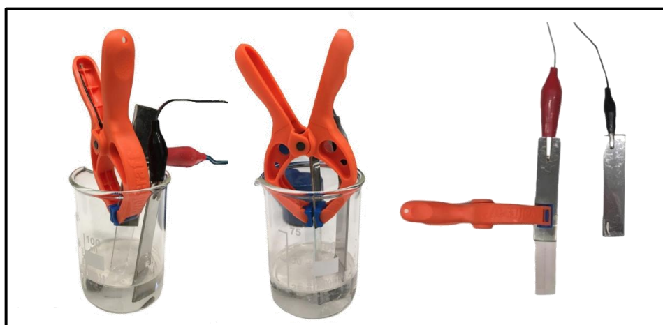
Figure 4.1.4.1.2. Electrochemical cell of Cyclic Voltammetry set-up used for the determination of Li + ions diffusion in a liquid electrolyte and in a gel polymer electrolyte.
