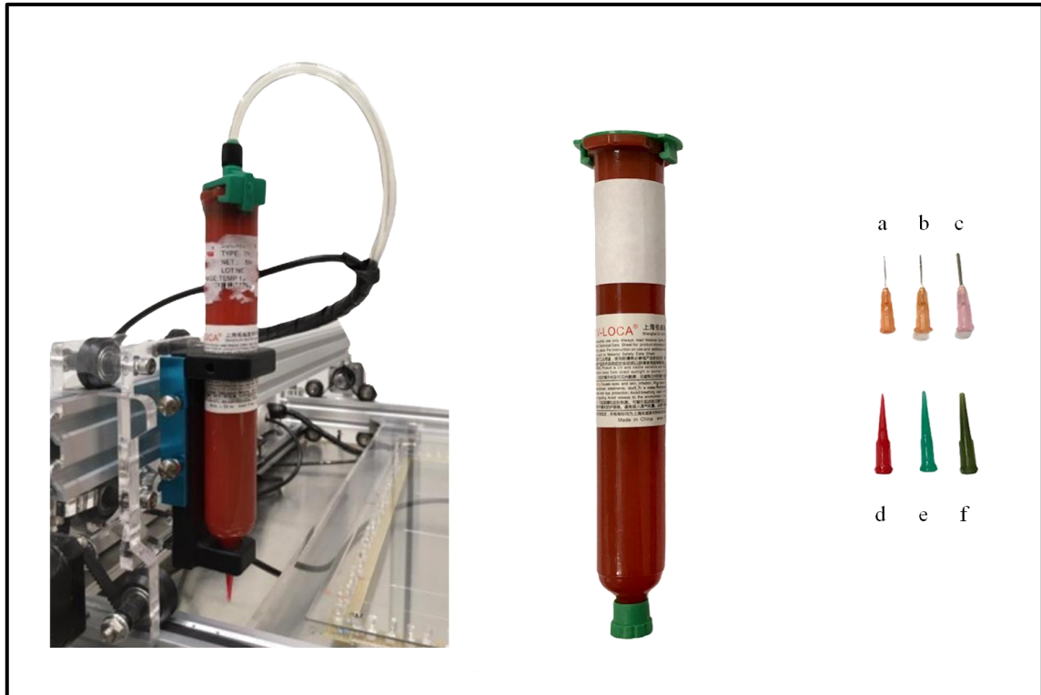
Figure 4.4.3.1.18. The Mobile Dosing Syringe, the UV-LOCA TP-2500F Glue and the available tips.
