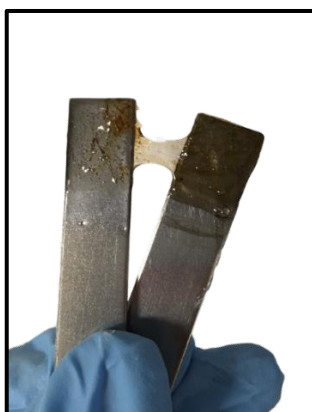
Figure 4.2.5.5. Instability of gel polymer electrolytes registered under high applied potential (over 4 V).
