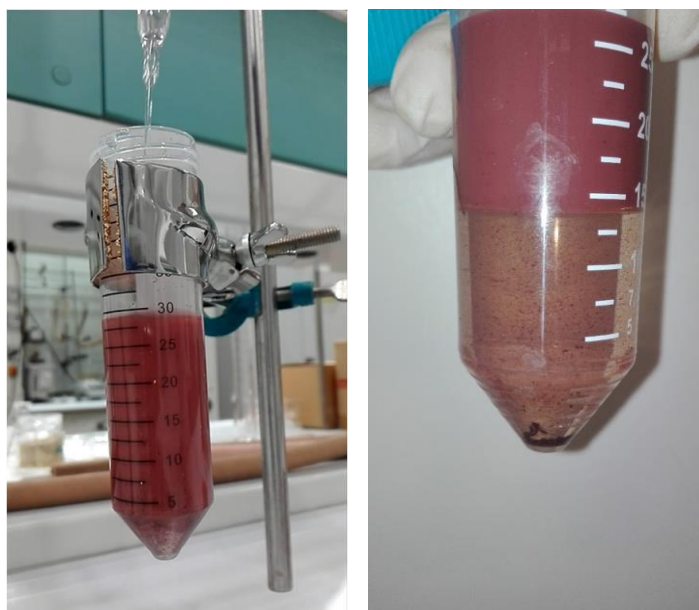
Figure 28 -The addition of \text{CHCl}_3 (left); the biphasic system with nanoparticles in water above and nanowires in chloroform below (right).
