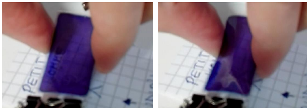
Figure 64 – Photographs of a device working without mechanical stress (left) and bent (right).
