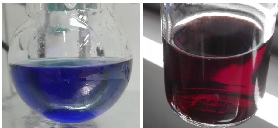
Figure 52 – Left: the freshly prepared film-forming solution, with double amount of TMPD. Right: the same solution degraded after a few days.
