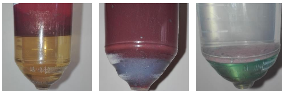
Figure 34 – CuNWs must be quickly extracted from CHCl 3 in order to avoid copper reoxidation phenomena, highlighted by the change in colour of the organic phase.
