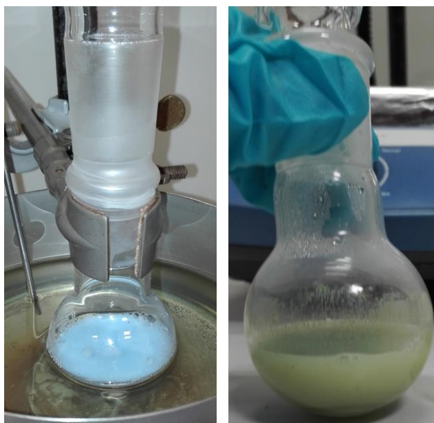
Figure 27 -If the same reaction is not closed and is carried out under reflux conditions through a condenser, it does not lead to the formation of CuNWs.
