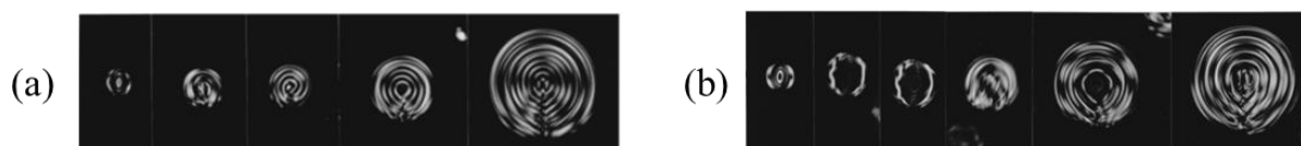
Figure 1.31 Cholesteric drop with a pitch of (a) p=7.4\mu\text{m} and the radii vary from 8.2 to 31.4\mu\text{m} (from left to right), and (b) p=17.7\mu\text{m} and the radii of the droplets varies from 11.5 to 41.0\mu\text{m} [9].
