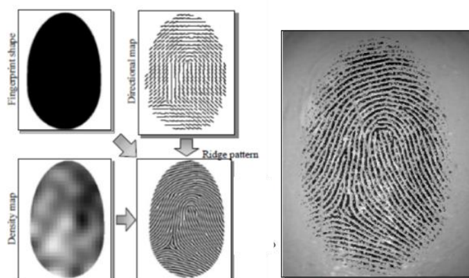
Figure 1. 46 Schematic representation of the four steps to create a synthetic fingerprint[61] (left) and a synthetic fingerprint image created with SFinGe approach (right).
