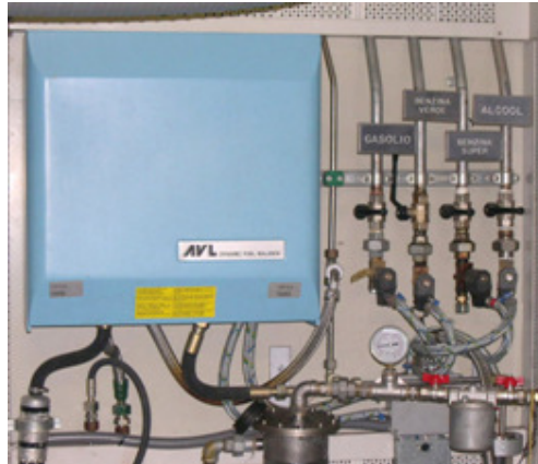
Fig. II.1.9.1– AVL dynamic fuel consumption system
