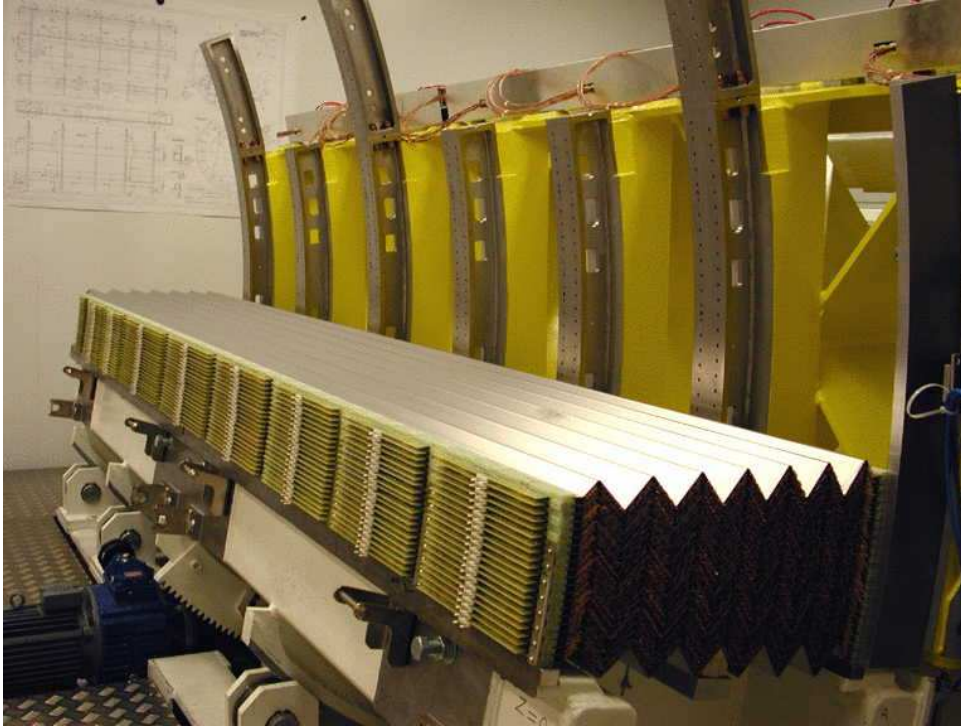
FIGURE 2.13: Photograph of a partly stacked barrel electromagnetic LAr module. The accordion structure is clearly visible. Photograph taken from [57].
