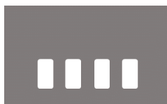
Figure 5.4- Metallic mask used to define active area during J-V measurements.
