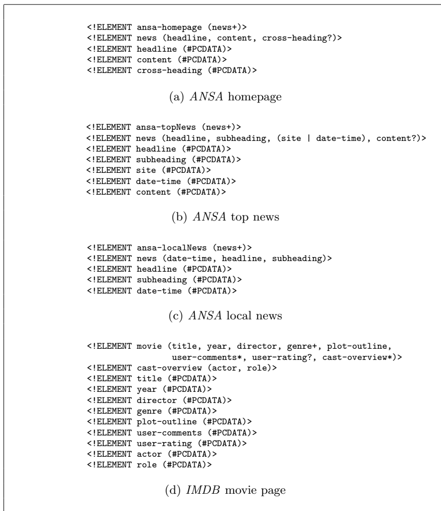
Fig. 3.13: Extraction schemas associated with the test sites
