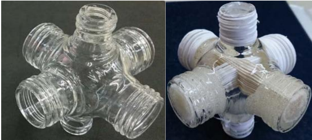
Fig 32. Bioreactor housing (left-a) and bioreactor assembled in-house, with 100 HFs (10x10 arrangement) in each bundle (right-b).
