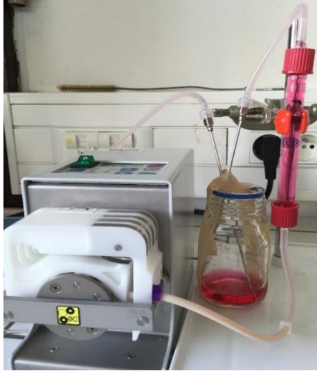
Fig. 14. Fluidized bed bioreactor used to study the transport of vitamin B12 into the beads (dynamic system)
