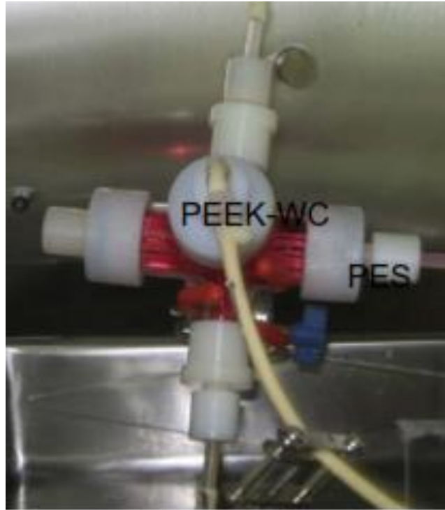
Fig. 28. Crossed hollow fiber membrane bioreactor
