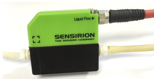
Fig 40. SENSIRION SLI 2000 flow meter.
