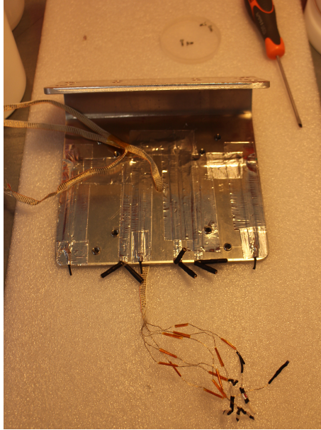
Figure 5.1: CORA support and control Aluminum plate with heaters installed
