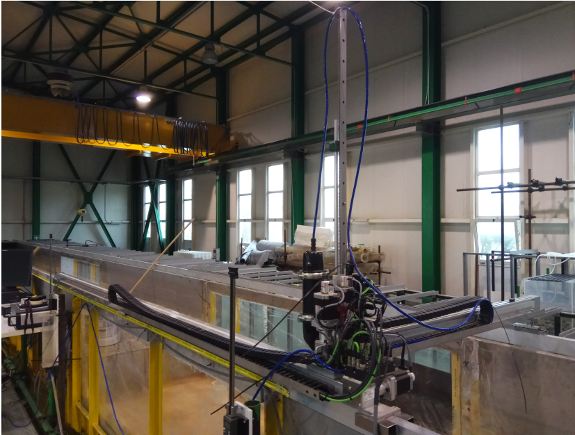
Figure A.1: Traverse System.
