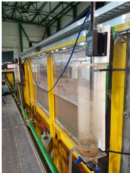
Figure 3.17: Piezometers equipment used to measure the water surface slope.
