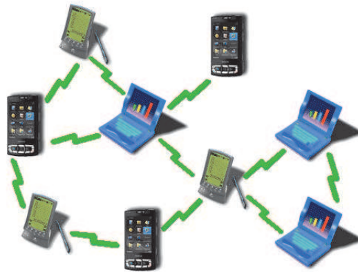
Fig. 2.1 An example of Mobile Ad-hoc Network scenario
