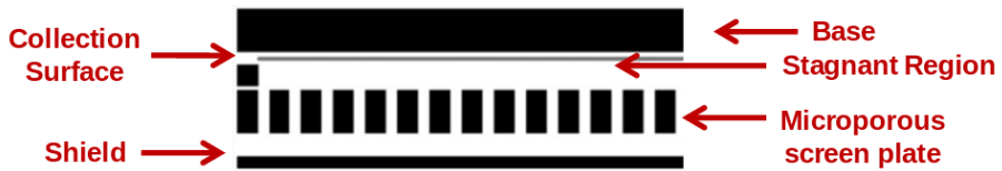
Figure 5.1: Simplified scheme of a passive sampler.
