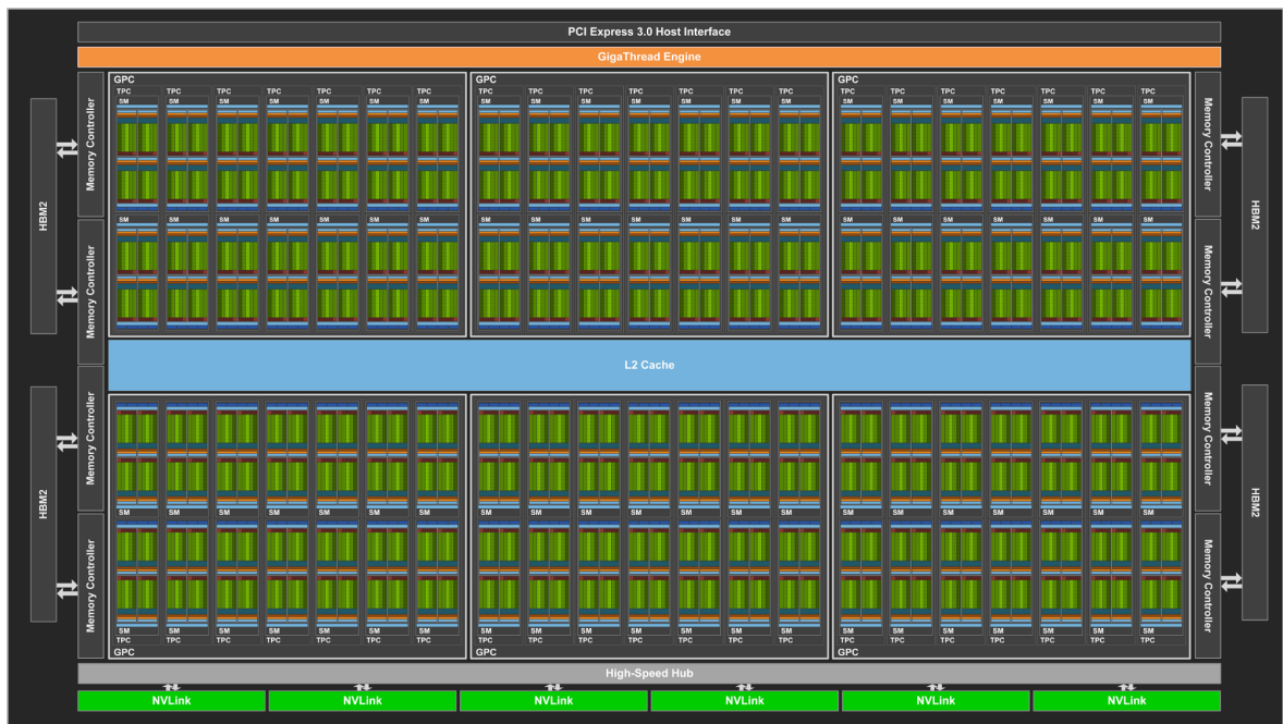
FIGURE A.3: Volta GV100 Full GPU with 84 SM Units.
