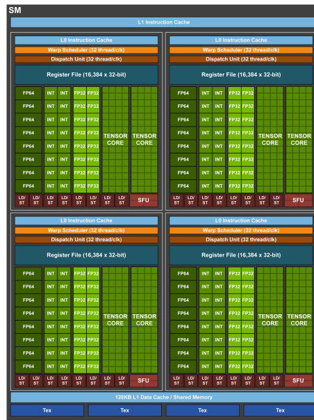
FIGURE A.2: NVIDIA GPU Volta SM Architecture.
