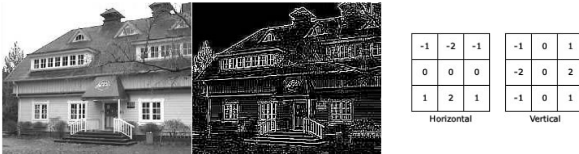
FIGURE 6.9: Sobel edge detection filter. The new pixel value is computed in two subsequent steps, horizontal and vertical, in order the final image to be less affected by noise.
