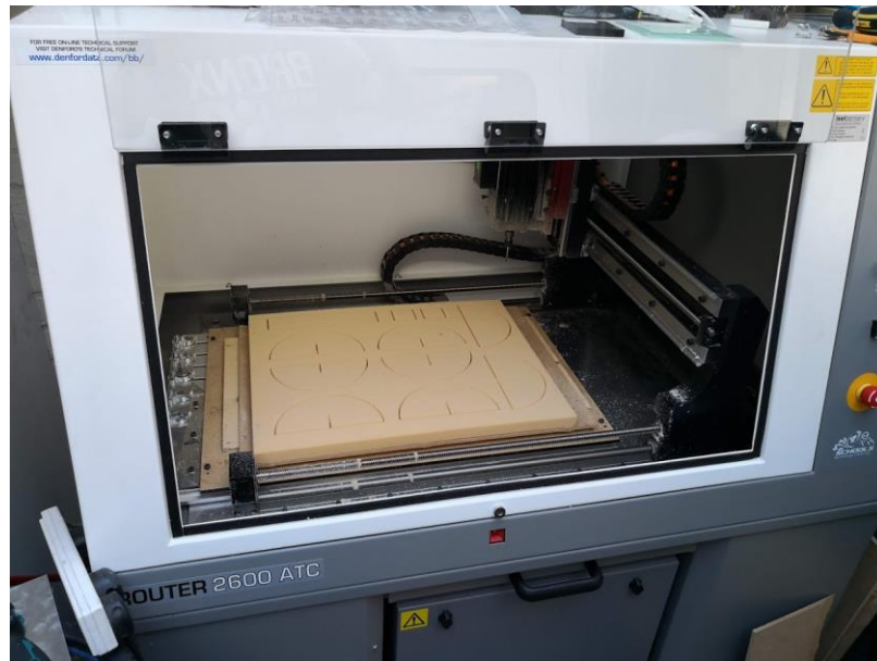
Fig. 4.39: Cutting samples by using Denford CNC router.
