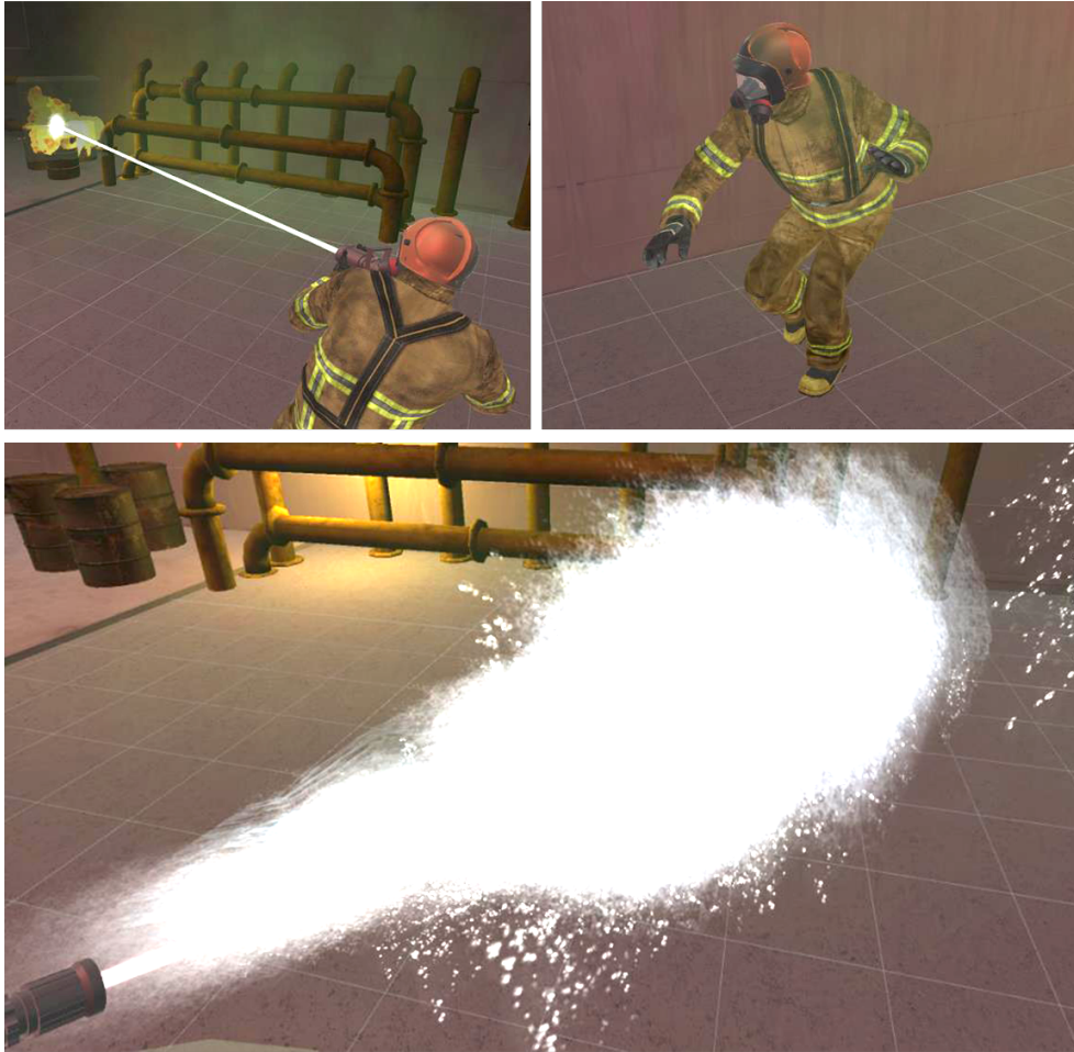
Figure 25: Using particle system technology for the fire extinguishing fluid
