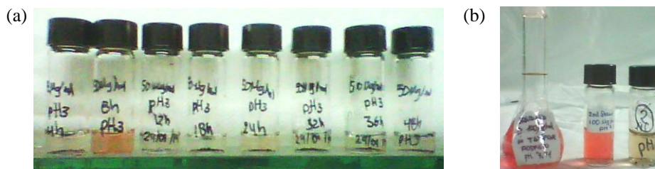
Figure 4.3 Increment of adsorption process at different pH (a) Test of DOX-GO at pH 3 in a concentration of 50 \mu\text{g/mL} , (b) test of DOX-GO at pH 7.7 in a concentration of 100 \mu\text{g/mL} .
