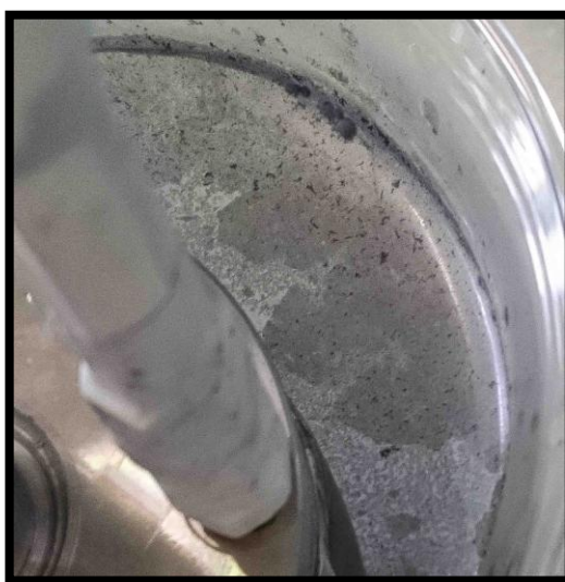
Figure 3.5 Material generated by arc discharge in the synthesis chamber.
