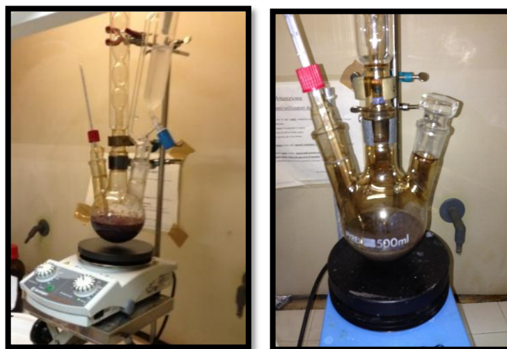
Figure 1.6 Pictures of the oxidation of graphite by chemical process. Left mixture of reagents with graphite and addition of peroxide water and on the right mixture after heating at 50^\circ\text{C} .
