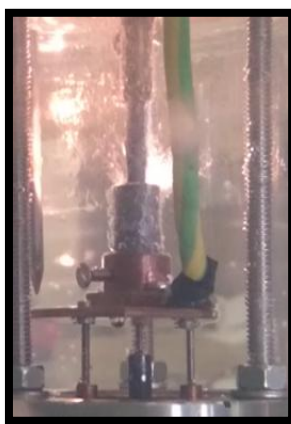
Figure 3.3 Digital image of the experimental process during arc discharge between anode and cathode of graphite.
