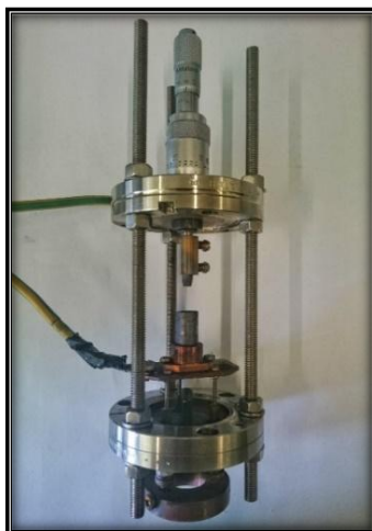
Figure 3.1 Apparatus assembled to synthesis of CNOs by arc discharge in water.
