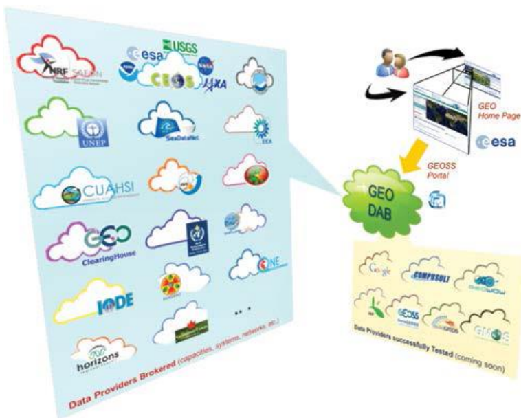
Figure 1 The GEOSS Portal enables discovery and access to the comprehensive data produced by the GEOSS community by connecting to the GEO-DAB, the broker (mediator) component in the GEOSS architecture.
