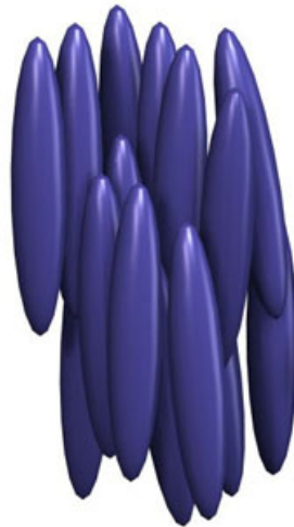
Figure 1.3: Liquid crystal in nematic phase - A schematic representing mesogens as ellipsoidal rods, oriented in roughly the same direction, shows conceptually what order in the nematic phase is like
