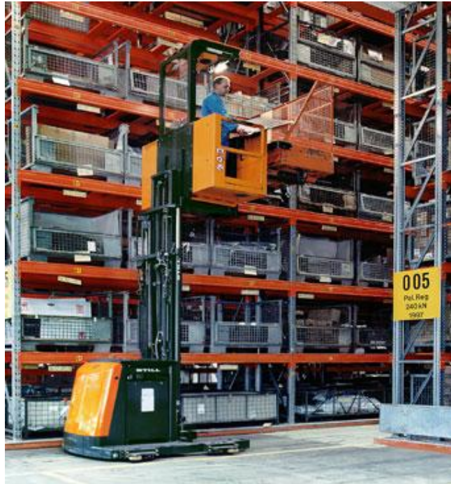
Figura 3.28 Carrello commissionatore verticale (Foto Still)
