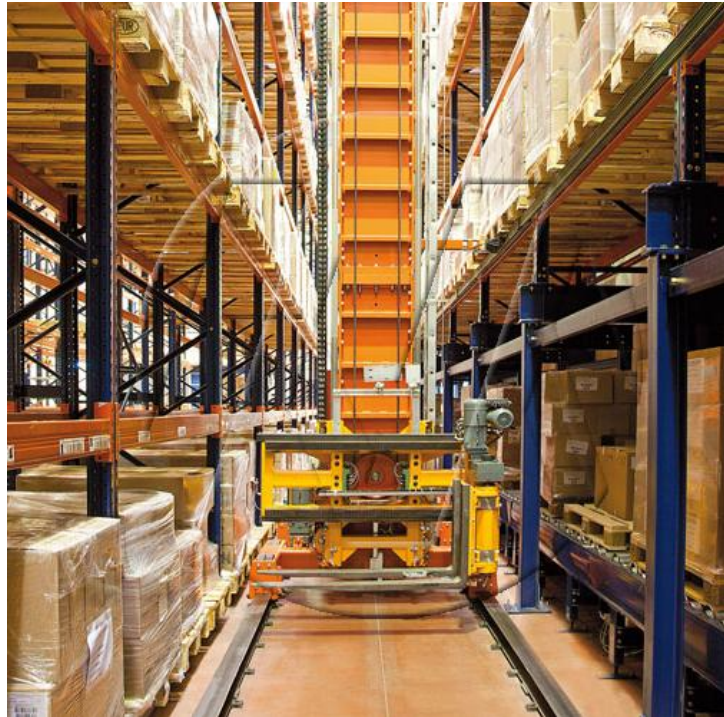
Figura 3.29 Trasloelevatori (Foto Mecalux)
